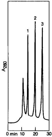
Fig. 6. Anion-exchange chromatography of nucleotides. Column: Hydrophase HP-PEI, 100 mm \times 6.5 mm. Sample: 1 = AMP; 2 = ADP; 3 = ATP. Temperature: ambient. Flow-rate: 1.0 ml/min. Detection: UV 280. Eluents: A = 10 mM Tris \cdot HCl (pH 7.5); B = A + 0.5 M sodium chloride; linear gradient from A to B in 10 min.
